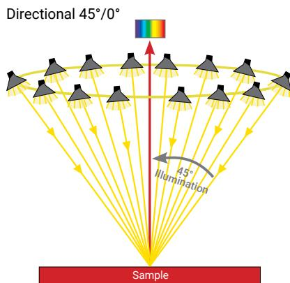
Regarding the sample shown on right, the diffuse geometry ( $d/8^\circ$ ), used in sphere instruments, will tell you that the sample is of the same color, no matter what the texture is. An instrument with the directional geometry ( $45^\circ/0^\circ$  or  $0^\circ/45^\circ$ ) will indicate that the four quadrants are different. Exactly just like your eye sees it. Which one is right then? That depends on your need.
